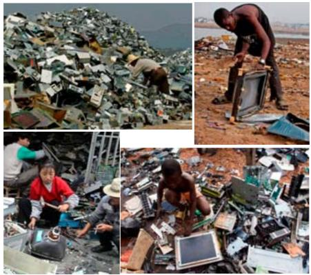
Figure 19: Collection, sorting and manual dismantling of electronic waste as it is performed in many developing countries, e.g. in China and Ghana (Photos: Top left: © Natalie Behring-Chisholm,Greenpeace, Bottom left: ©2006 Basel Action Network, Top right and bottom right: © Kate Davison, Greenpeace).
