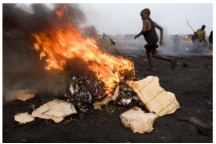
Figure 23. Burning of e-waste directly on the on the ground to recover valuable metals, Accra, Ghana (Photo: © Kate Davison, Greenpeace).
