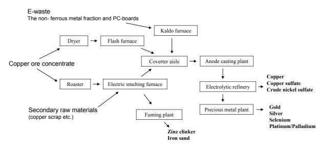
Figure 18. Schematic of the processes used to recover copper and precious metals from ore concentrate, copper scrap and e-waste at Boliden's Rönnskär smelter in Sweden [Boliden 2010].
