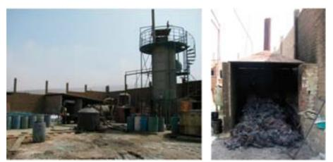
Figure 26. Simple facility for recycling of copper cables, showing the whole facility to the left and the cable burning furnace to the right. Ash sample 1 was collected here (Photos: © Viktor Sjöblom).
