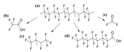
Figure 16. Molecular structures of the PTFE-polymer (a), and and a selction of its thermal decomposition products; (b) trifluoroacetic acid (TFA), (c) perfluorobutane (PFB), (d) perfluorooctanoic acid (PFOA), and (e) carbonyl fluoride (COF2).
