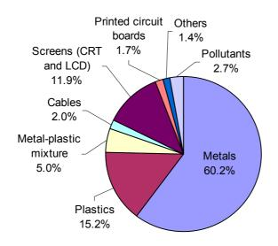
Figure 3. Average composition of materials found in e-waste according to the Swiss Federal Laboratories for Materials Testing and Research for industry (Empa), [Widmer et al 2005].
