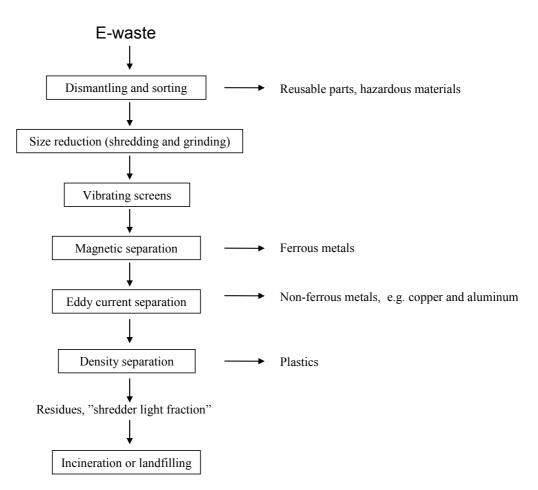
Figure 17. Schematic of the first steps in a typical e-waste recycling process.
